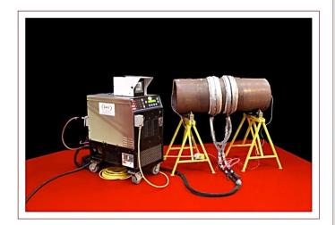
Cable identification system knows the type of cable attached and limits output to protect cables and blankets.
